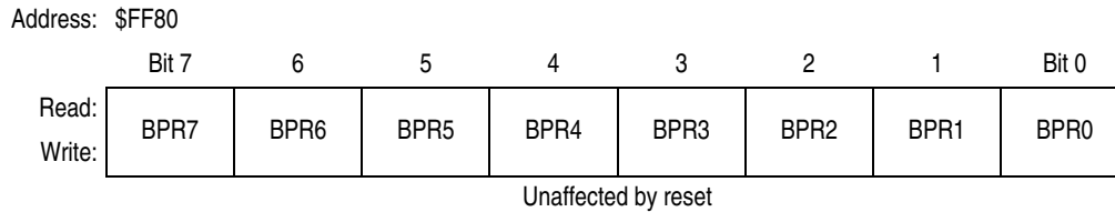
Figure 2-4. FLASH-1 Block Protect Register (FL1BPR)
