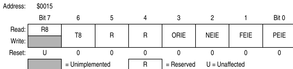
Figure 13-12. ESCI Control Register 3 (SCC3)
